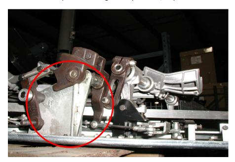
If this bracket assembly is silver in color, you have the original 90XL style as shown in the photo above. If the bracket is black in color, you have the newer XII style tie rod bracket assembly (as shown to the left).
